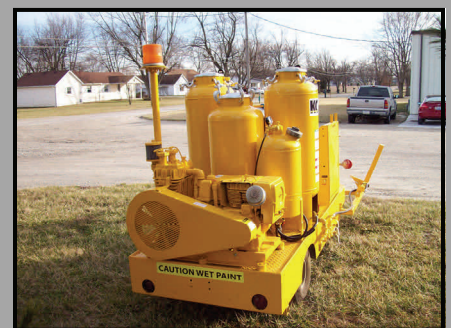
Kohler 12 HP gasoline engine Quincy 240 compressor with unloader
