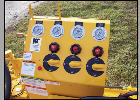
Operators control console with air regulators and gauges
