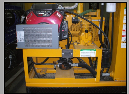
20 HP Honda Engine 13.1 CFM Quincy Compressor
