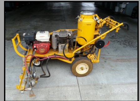
Honda 8 HP Engine and 18 CFM Two Stage Air Compressor
