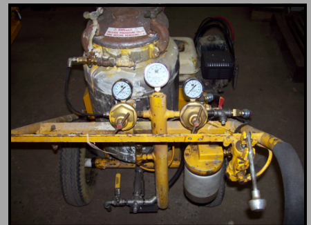
NEW Gauges, Rebuilt Regulators and QAW Valve
