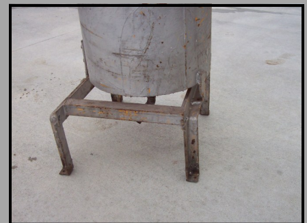
Tank is bolted to stand to accommodate lower plumbing
