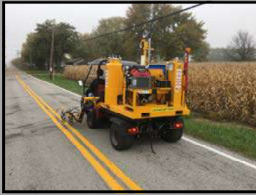
Self contained center & edgeline striper
