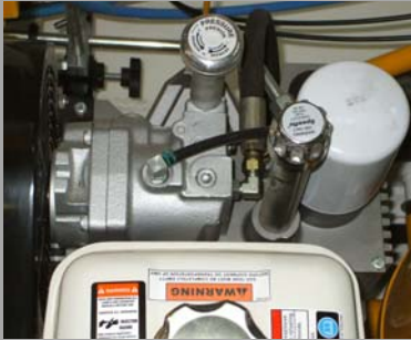
Hydraulic powered airless paint system
