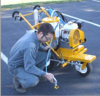
Detachable spray gun for remote work
