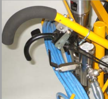
Exclusive "squeeze & lock" gun activator
