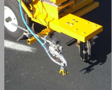
Heavy duty front locking swivel wheel
