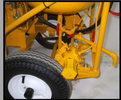
KC air actuated traction drive
